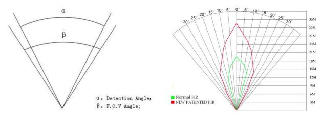
This camera has a new, patented design of the PIR. The new patented PIR's detection range can reach to 100ft (in good environments). The previous picture shows the compared detection zone between normal PIR and the new patented PIR.
