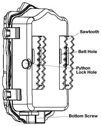
Fig. 6: The back panel of the camera
