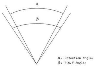
Fig.8: Detection angle vs. FOV angle
